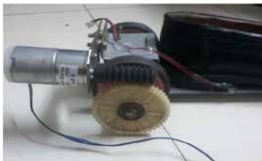
Fig. 7: Motor and Wheels Attached
